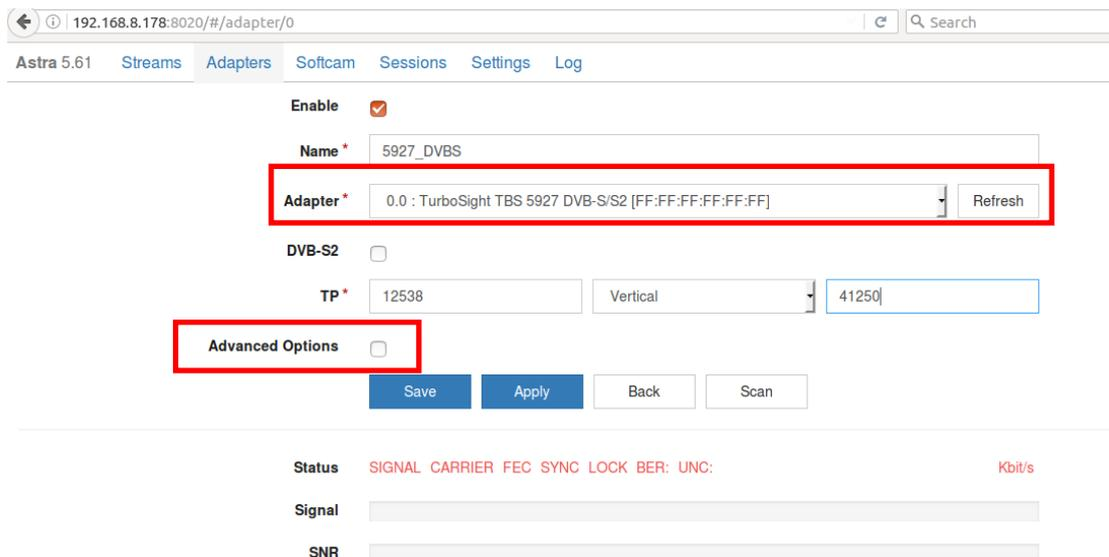
9.5 Then click “Scan” button to scan the channel, the sequence can not be reversed. After scanned out, select the channels you want and save, like this:
